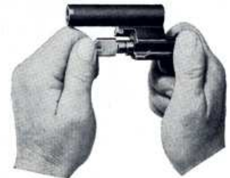
Fig. 35 Stripping the bolt assembly
