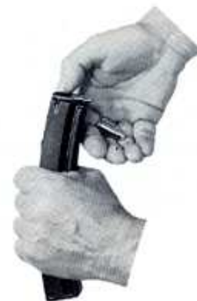
Fig. 24 Emptying the magazine
