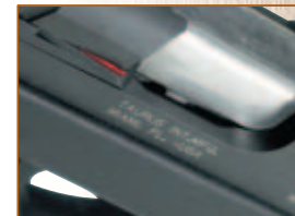
The Millennium Features a Loaded Chamber Indicator.
